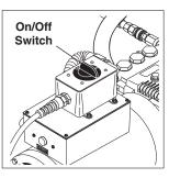
**STEP 2:** Turn off machine by turning switch to "OFF" switch.
