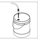
STEP 1: Remove detergent suction tube from container and insert into one gallon of fresh water. Slide nozzle forward for low pressure or use black detergent nozzle. Pull trigger on spray gun and siphon fresh clean water for one minute.
