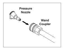
**STEP 6:** Pull spring-loaded collar of the wand coupler back to insert your choice of pressure nozzle.
