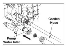
**STEP 10:** Check inlets filters, remove debris, then connect the garden hose to pump water inlet. *CAUTION: Do not run the pump without water or pump damage will result.*
