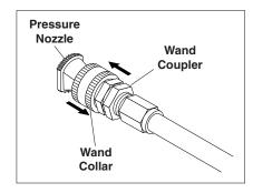
**STEP 6:** Pull the spring-loaded collar of the wand coupler back to insert your choice of pressure nozzle. Release the coupler collar and push the nozzle until the collar clicks. Pull the nozzle to make sure it is seated properly.
