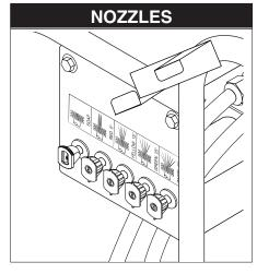
The five color-coded quick connect nozzles provide a wide array of spray widths from 0° to 40° and are easily accessible when placed in the convenient rubber nozzle holder, which is provided on the front of the machine.
