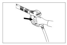
**STEP 3:** Press trigger to release water pressure.
