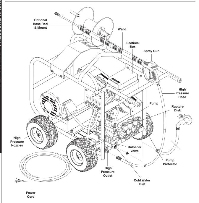
**Pump** — Delivers a specific gpm to the high pressure nozzle which develops pressure.
