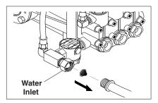
**STEP 4:** Disconnect the garden hose from the water inlet on the machine.
