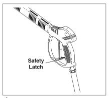
AWARNING! Never replace nozzles without engaging the safety latch on the spray gun trigger.
