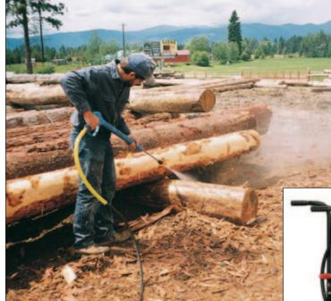
Stripping bark from logs is only one of the many applications for the MP or MPE high-pressure washers with cleaning power of up to 5,000 PSI.
